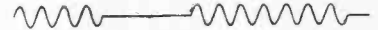
Fig. 3. Sample of carrier wave interrupted by morse keying. Here the carrier cycles that remain are identical with those in Fig. 1, so where do side frequencies come in?
